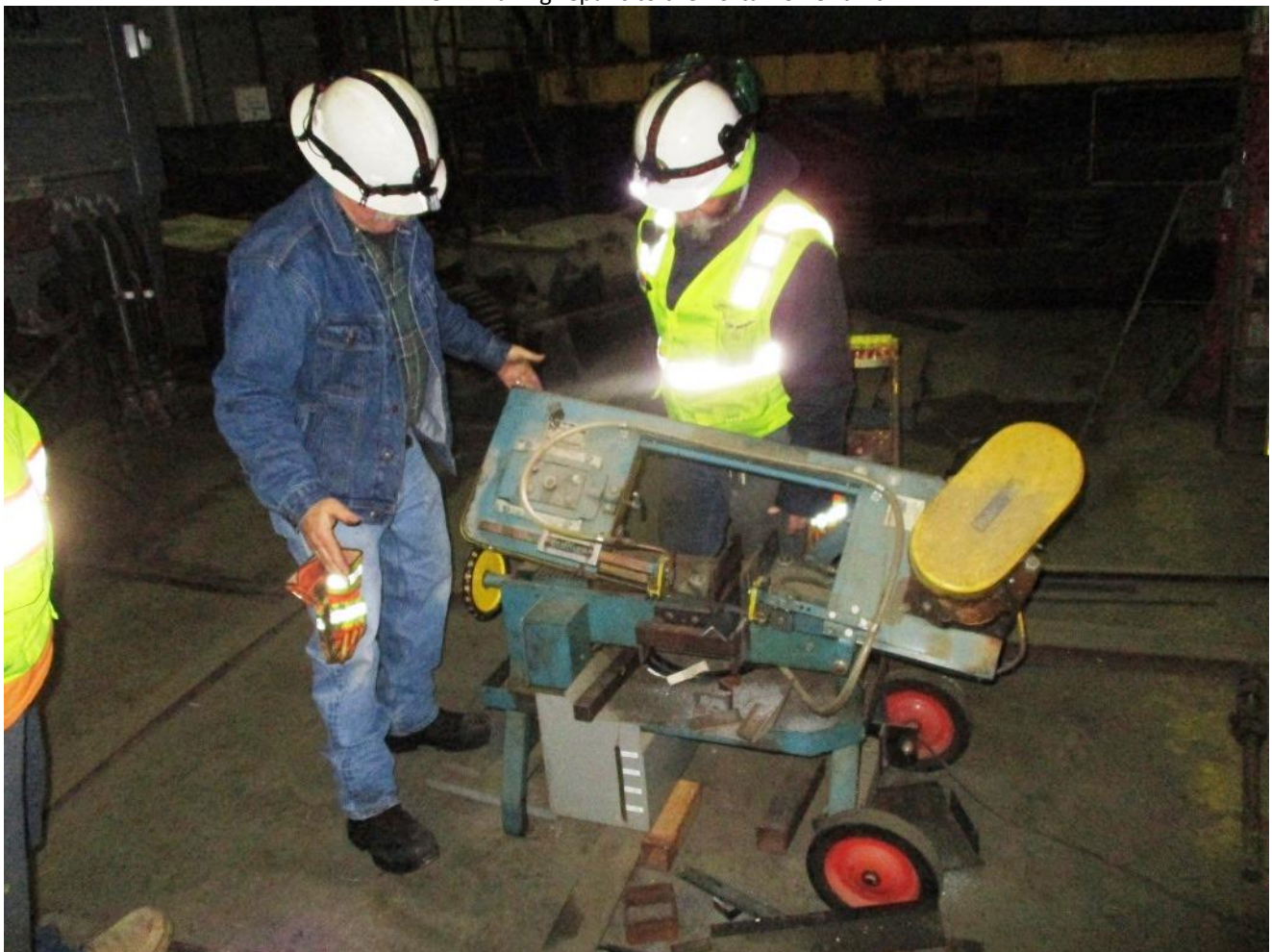
Mike H. and Joe cutting angle-iron to use as hasps to lock the red-flag in the retracted position
