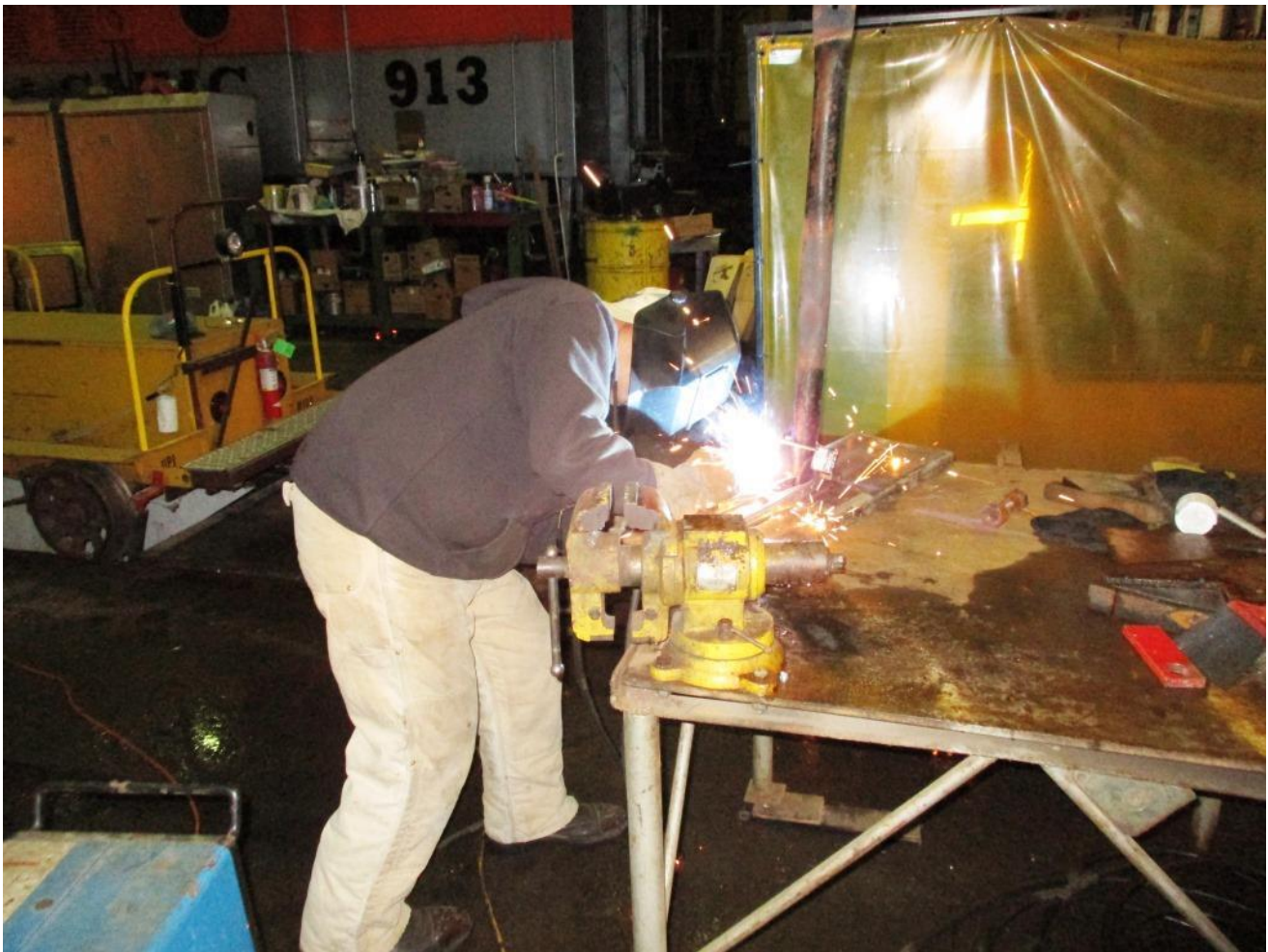
Cliff welding the locking hasp onto the retractable red-flag
